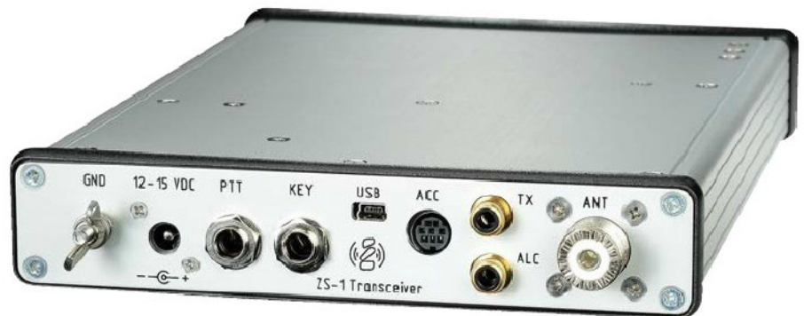
Figure 1 — The ZS-1 rear panel has connections for interfacing with a computer, external power amplifier, antenna, and station accessories.
