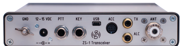
PHOTO 2: Zeus ZS-1 interconnections on the rear panel.
